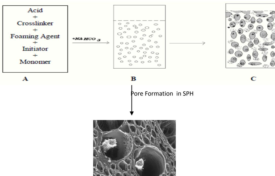
Fig 2: Schematic representation of the superporous hydrogel preparation[16].
